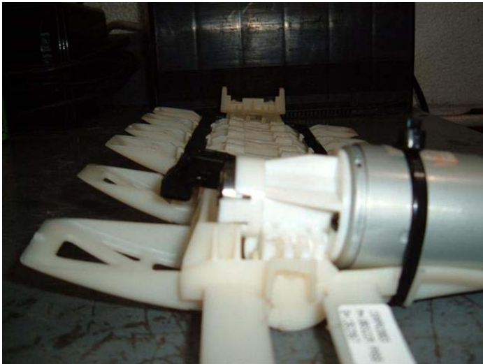
This is what happens when there's no retainer or clamp for the motor (Notice bearing slipping out of clips and motor tilted)
